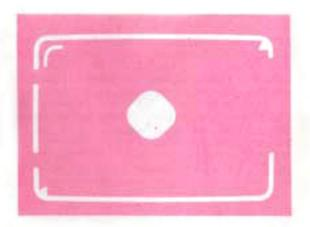
B. If the exposure warning lamp at the upper right-hand frame lights and then goes out as you continue to depress the shutter release button, a shutter speed of 1/30 sec. or slower is indicated, and use of a tripod is recommended if you are not using flash. Your Hi-matic F will continue to make accurate auto exposures down to 4 full seconds without flash. Adequate attention should of course be paid to subject movement at slow shutter speeds.
