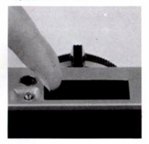
2. Making sure the end of the clear vinyl strip is projecting from the end of the compartment near the cover hinge, insert the 2 batteries as indicated by the diagrams in the bottom of the compartment. Then close and latch cover by holding it down and sliding it in the direction of the arrow, then letting it snap back in the opposite direction.
