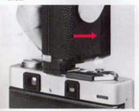
If you use a flash unit such as the regular Minolta Electroflash, which has a sync. cord, be sure to connect the plug of the flash cord with the sync. terminal of the camera as well.
