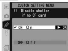
Highlight **f7 No CF card?** in the second level of the CSM menu (178) and press the multi selector to the right. Press the multi selector up or down to highlight an option, then press to the right to make a selection.
