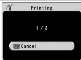
Begin printing. To cancel and return to PictBridge menu before all images have been printed, press button again. Turn camera off and disconnect USB cable when printing is complete.
