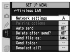
**Network settings:** Adjust settings for connection to a wireless network. Press the multi selector up or down to highlight an option and then press the multi selector to the right.
