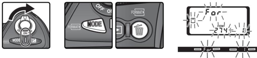
During formatting, the letters **F o r** will appear in the frame-count display. When formatting is complete, the frame-count display will show the number of photographs that can be recorded at current settings.
