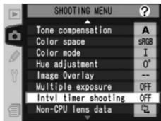
2 Press the multi selector left or right to highlight options and press the multi selector up or down to change interval timer settings. The selected option is highlighted in blue. The following options are available:
