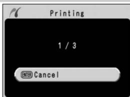
Begin printing. To cancel and return to PictBridge menu before all images have been printed, press **Enter** button again. Turn camera off and disconnect USB cable when printing is complete.
