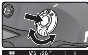
When matrix metering is selected, the metering display in the viewfinder shows **[M]**.
