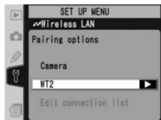
Press the multi selector up or down to highlight an option and then press the multi selector to the right.
