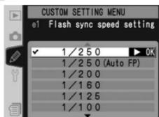
Highlight **e1 Flash sync speed** in the second level of the CSM menu (178) and press the multi selector to the right. Press the multi selector up or down to highlight an option, then press to the right to make a selection.
