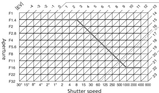
The maximum and minimum values for EV vary with sensitivity (ISO equivalency); the above graph assumes a sensitivity of ISO 100 equivalent. When matrix metering is used, values over  $16\frac{2}{3}$  EV are reduced to  $16\frac{2}{3}$  EV.
