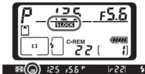
6 Recompose the photograph and press the shutter-release button the rest of the way down to shoot. If desired, additional pictures can be taken without releasing FV lock.
