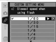
Highlight **e2 Flash shutter speed** in the second level of the CSM menu (178) and press the multi selector to the right. Press the multi selector up or down to highlight an option, then press to the right to make a selection.
