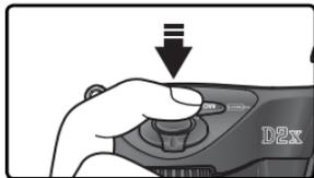
**5** Press the shutter-release button the rest of the way down to acquire Image Dust Off reference data (note that noise reduction turns on automatically when the subject is poorly lit, increasing the amount of time needed to record the data). The monitor turns off when the shutter-release button is pressed.
