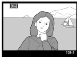
To remove protection from the photograph so that it can be deleted, display the photograph or highlight it in the thumbnail list and then press the
