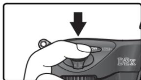
In single-servo AF, focus will remain locked between shots as long as the shutter-release button is kept pressed halfway, allowing several photographs in succession to be taken at the same focus setting. Focus will also remain locked between shots while the **AE-L/AF-L** button is pressed.
