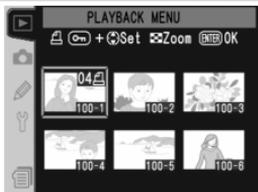
Press button and press multi selector up or down to specify number of prints (up to 99), or press center of multi selector to select image and set number of prints to 1. Selected images are marked by icon.
