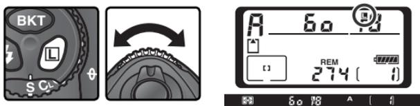
To unlock aperture, press the **L** button and rotate the sub-command dial until the lock icons disappear from the displays.
