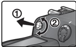
Diopter can be adjusted in the range  $-3\text{ m}^{-1}$  to  $+1\text{ m}^{-1}$ . Corrective lenses (available separately; Ⓜ 244) allow diopters of  $-6\text{ m}^{-1}$  to  $+3\text{ m}^{-1}$ .
