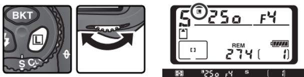
To unlock shutter speed, press the **L** button and rotate the main command dial until the lock icons disappear from the displays.
