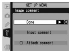
Highlight **Image comment** in the setup menu (📖 209) and press the multi selector to the right. Press the multi selector up or down to highlight an option, then press to the right to make a selection.
