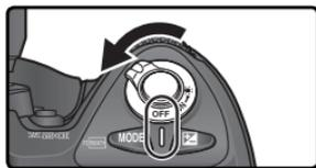
**2** Open the cover protecting the A/V-out and DC-in connectors.
