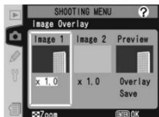
**5** Press the multi selector up or down to select a value for gain between 0.1 and 2.0. The default value is 1.0; selecting 0.5 cuts gain in half, while selecting 2.0 doubles gain. The effects of gain are visible in the preview image.
