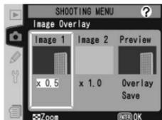
**6** Press the multi selector left or right to highlight **Image 2**. Repeat steps 3–5 to select the second image and adjust gain.
