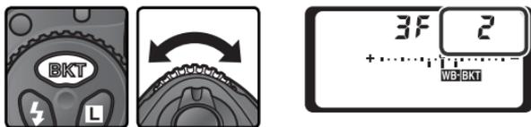
**4** Compose a photograph, focus, and shoot. Each shot will be processed to create the number of copies specified in the bracketing program, and each copy will have a different white balance. Modifications to white balance are added to the white balance adjustment made with white balance fine-tuning (🔍 56).
