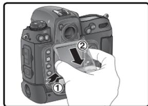
To replace the cover for shooting or storage, insert the two projections on the top of the cover into the matching indentations above the camera monitor (1), then press the bottom of the cover until you hear it click into place (2).
