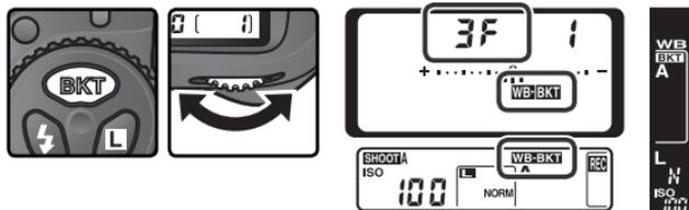
If the number of shots in the bracketing program is greater than the number of exposures remaining, a flashing icon will appear in the top control panel and the frame count and number of exposures remaining will flash. A flashing indicator will appear in the viewfinder and the shutter release will be disabled. Shooting can begin when a new memory card is inserted.
