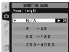
4 Select the lens focal length (in mm) and press the multi selector to the right.
