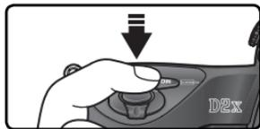
While the photograph is being recorded to the memory card, the access lamp next to the card slot cover will light. **Do not eject the memory card, turn the camera off, or remove or disconnect the power source until the lamp has gone out.** Removing the memory card or cutting power in these circumstances could result in loss of data.
