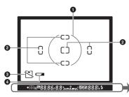
When the battery is totally exhausted, the display in the view-finder will dim. The view-finder display will return to normal when a fully-charged battery is inserted.
