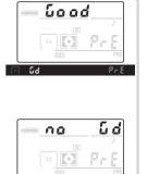
If lighting is too dark or too bright, the camera may be unable to measure white balance. A flashing no unable to measure white balance. A flashing no unable distribution of the control panel and viewfinder. Return to Step 4 and measure white balance again.
