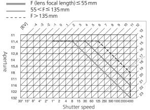
The maximum and minimum values for EV vary with sensitivity (ISO equivalency); the above graph assumes a sensitivity of ISO 200 equivalent. When matrix metering is used, values over 17½ EV are reduced to 17½ EV.
