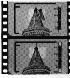
RANGE FINDER. While sighting through the VIEWFINDER rotate the FOCUSING RING until the double image, visible in the center of the field, is super-imposed. This brings picture into perfect focus and is particularly important when taking FLASH pictures.
