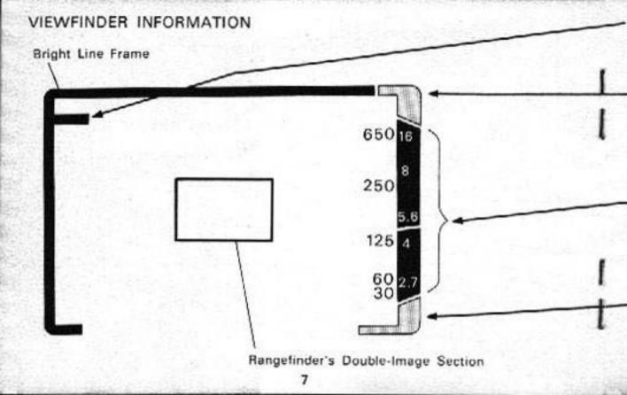
PARALLAX MARKS. When taking pictures closer than four feet from camera, subject should not extend above the PARALLAX MARK.
