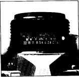
The figures seen in the viewfinder from "2" to "2000" refer to the shutter speeds in fractions of seconds (i.e., 1/2 sec. to 1/2000 sec.), "1" to "4S" indicate full-second shutter speeds.
