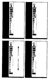
Shutter Speed First: Set the desired shutter speed with the shutter speed control pushbuttons. If the "OVER" LED still flashes, stop the lens down to a smaller aperture (i.e., f/5.6 to f/11, f/16, etc.) until it goes out. If the "UNDER" LED remains lit, set the lens to a wider aperture (i.e., f/5.6 to f/2, f/1.4, etc.). Exposure is correct when the shutter speed and the "M" LED are the only LEDs that remain lit in the viewfinder.
