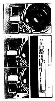
**EXPOSURE SETTING:** With the manual exposure system you have the option of setting either the shutter speed or the lens aperture first. The "OVER and "UNDER" LEDs flash in the viewfinder to serve as guides for setting the correct exposure.
