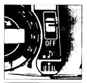
Audio Focus Indication: The ME-F provides you with an audible signal which accompanies the LED correct focus indicator. This signal tells you when to take the picture. To operate the audio focus indicator, set the audio focus switch to the musical note. When not needed, turn the audio focus indicator off simply by sliding the switch from the musical note back to the black square.
