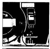
Audio Focus Indication: The ME-F provides you with an audible signal which accompanies the LED correct focus indicator. This signal tells you when to take the picture. To operate the audio focus indicator, set the audio focus switch to the musical note. When not needed,turn the audio focus indicator off simply by sliding the switch from the musical note back to the black square.
