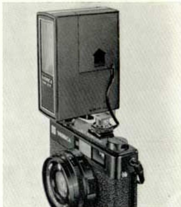
When using film with speed ratings other than those indicated in this section, or when photographing subjects closer than or beyond the specified EZ-flash range, the correct aperture setting must also be obtained by dividing the guide number by the camera-to-subject distance.
